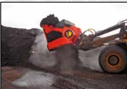
Aerating sludge compost
