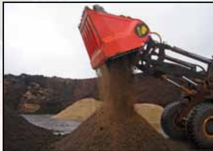
Mixing top soil and sand
