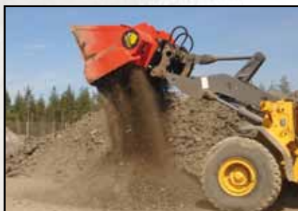
Aerating contaminated soil compost
